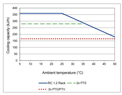
Note: The limit curves for the heat exchangers exchanger apply to a dew point of 40  $^{\circ}\text{C}.$
