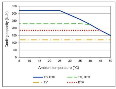
Remark: The limit curves for the heat exchangers exchanger apply to a dew point of 65 °C.
